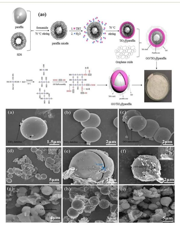
Fig. 14 (a0) Schematic illustration of the method for creating  $GO/TiO_2$ /paraffin microcapsules, SEM images of (a and b)  $TiO_2$ /paraffin microcapsules, (c and d)  $GO/TiO_2$ /paraffin microcapsules containing 1 wt% GO, (e-g)  $GO/TiO_2$ /paraffin microcapsules containing 2 wt% GO, and (h and i)  $GO/TiO_2$ /paraffin microcapsules containing 3 wt% GO. Reproduced with permission from ref. 163 Copyright 2021 Elsevier.
