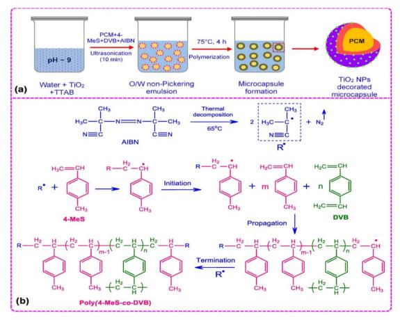
Fig. 7 (a) Schematic illustration for the creation of a crosslinked polystyrene-based shell decorated with TiO<sub>2</sub> nanoparticles and (b) free radical polymerization for the creation of the poly(4-methylstyrene-co-divinylbenzene) shell.<sup>47</sup> Reproduced with permission from ref. 47. Copyright 2021 ACS.
