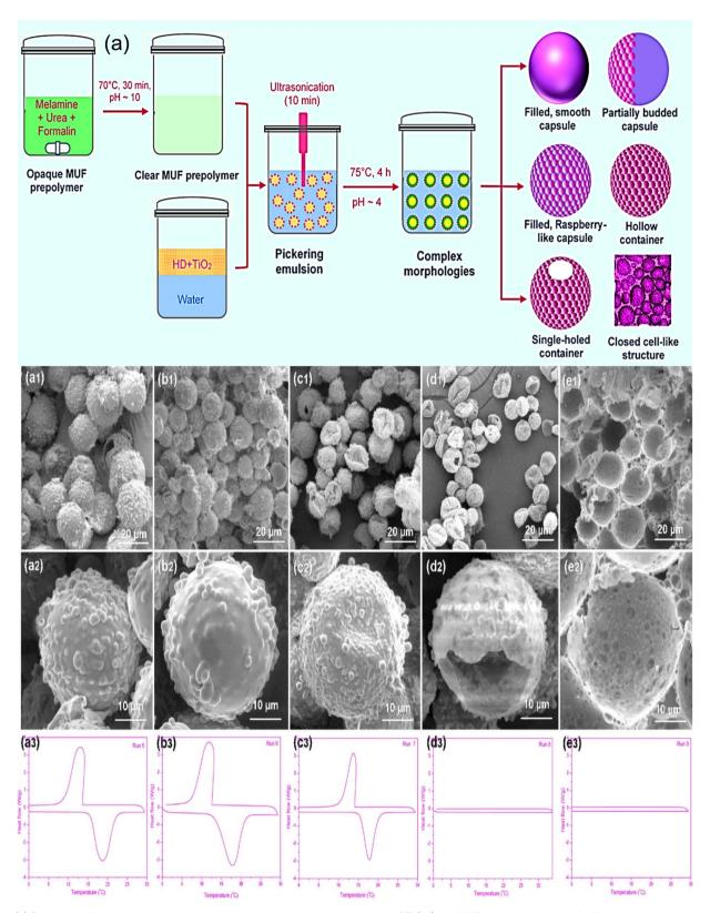
Fig. 5 (a) Schematic illustration steps involved in creating a complex structure of  $TiO_2$ /polyMUF microcapsules with distinct morphologies, DSC thermograms, and SEM images of the microcapsules at different core-to-shell ratios, (a1–a3) core-to-shell ratio of 1:2, (b1–b3) core-to-shell ratio of 1:1, (c1–c3) core-to-shell ratio of 1:0.5, (d1–d3) core-to-shell ratio of 1:5:1, and (e1–e3) core-to-shell ratio of 2:1. Performance with permission from ref. 141 Copyright ACS 2022.
