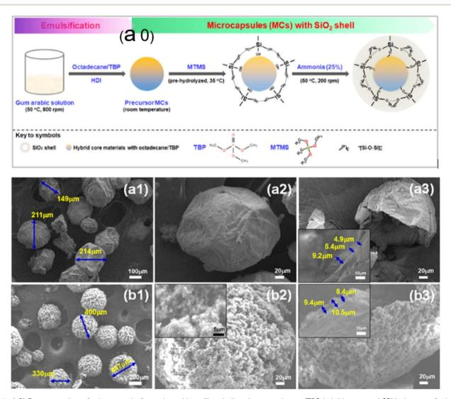
Fig. 13 (a0) Representation of microcapsule formation with a silica shell and an octadecane/TBP hybrid core, and SEM pictures of a hybrid MEPCM with SiO<sub>2</sub> (a1-a3) and PUF (b1-b3).<sup>2</sup> Reproduced with permission from ref. 2 Copyright 2021 ACS.
