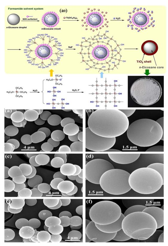
Fig. 15 (a0) Schematic illustration of the fabrication of the n-eicosane microcapsule TiO<sub>2</sub> shell, SEM images of the n-eicosane microcapsule (a and b) produced with a weight ratio of 60/40 n-eicosane/TBT, (c and d) produced with a weight ratio of 50/50 n-eicosane/TBT, and (e and f) produced with a weight ratio of 40/60 n-eicosane/TBT. Reproduced with permission from ref. 129 Copyright 2015 Elsevier.
