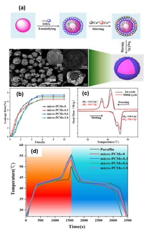
Fig. 19 (a) Schematic of synthesis for paraffin microcapsules composed of Ce<sup>3+</sup> dopped calcium carbonate with SEM images; (b) Leakage rate of paraffin microcapsules; (c) DSC curves of PCM microcapsules containing 0.6 wt% Ce<sup>3+</sup> with respect to calcium carbonate; (d) paraffin and paraffin microcapsules' temperature – time curves during the release processes (blue) and storage (red). <sup>177</sup> Reproduced with permission from ref. 177 Copyright 2019 ACS.
