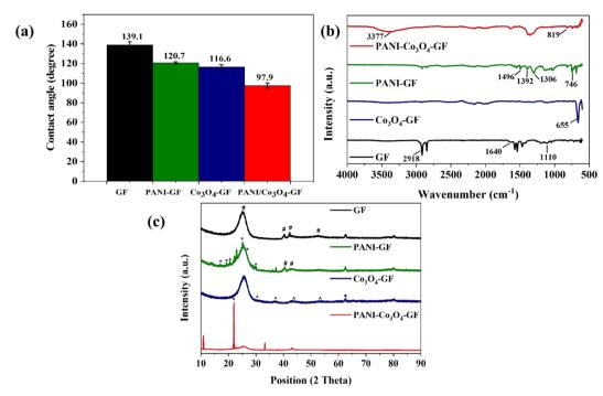
Fig. 2 Physicochemical analyses of the four anodes tested in this study. (a) Contact angle measurements, error bars account for the deviation in the measured angle at three different points on the electrode surface. (b) FTIR spectra. (c) XRD analysis.
