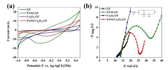
Fig. 4 Electrochemical characterisation of the anode electrodes before use. (a) CV scans at 0.01 V s<sup>-1</sup> and (b) EIS spectra. Tests were performed in a 3-electrode system in 50 mM PBS (pH 7), with the anode as the working electrode and Pt wire (diameter: 0.127 mm) as the counter electrode.
