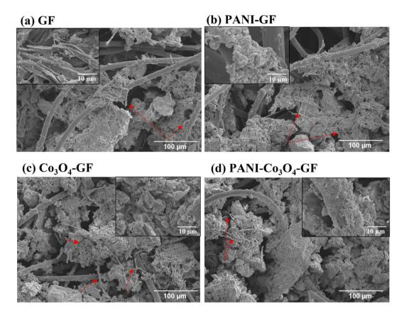
Fig. 9 SEM images of after 4 months of operation of the anodes: (a) GF, (b) PANI–GF, (c)  $Co_3O_4$ –GF, and (d) PANI– $Co_3O_4$ –GF. Images were taken at 10 kV, with magnification 300. Red arrows in the images indicate filamentous assemblies.
