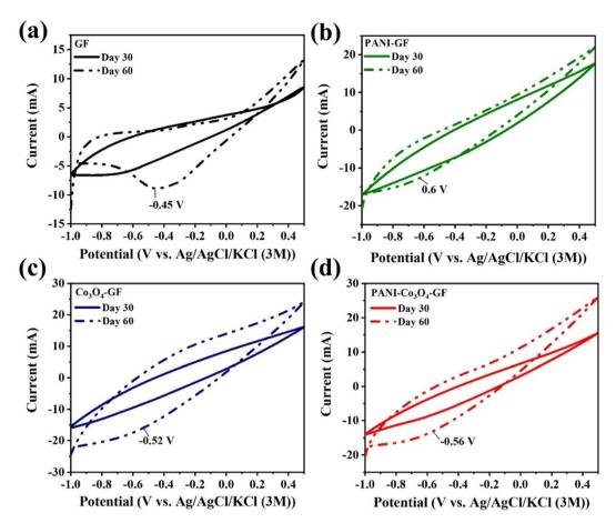
Fig. 5 Comparison of CV scans at  $0.01 \text{ V s}^{-1}$  obtained with the anode tested in SMFCs operated for 30 and 60 days. (a) GF; (b) PANI–GF; (c)  $Co_3O_4$ –GF; (d) PANI– $Co_3O_4$ –GF. Values are averages calculated from 3 replicate anodes with a maximum standard deviation of  $\pm 6.1$  mA,  $\pm 2.4$  mA,  $\pm 4.5$  mA and  $\pm 4$  mA, respectively.
