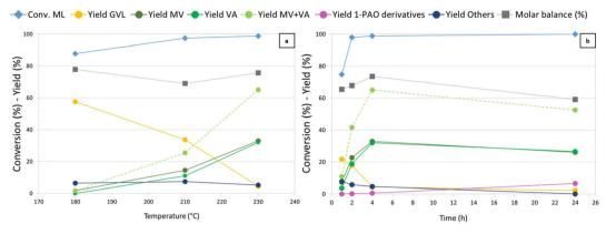
Fig. 2 ML hydrogenation over Re-Ru-O/HZSM-5. Reaction conditions: solvent free (ML neat),  $P_{H2} = 40$  bar, catalyst loading = 5 wt%  $[m_{cat}/m_{ML}]$ . (a) Effect of temperature for a 4 h reaction time and (b) effect of reaction time at 230 °C. Others = 2-MTHF, 4-HPA/E and unidentified products.
