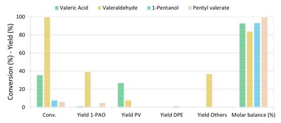
Fig. 5 Investigation of the reaction pathway loading intermediates and products in the presence of Re-O/SiO<sub>2</sub>. Reaction conditions: solvent free, T = 210 °C,  $P_{H2} = 40$  bar, t = 4 h, catalyst loading = 5 wt%  $[m_{cat}/m_{reactant}]$
