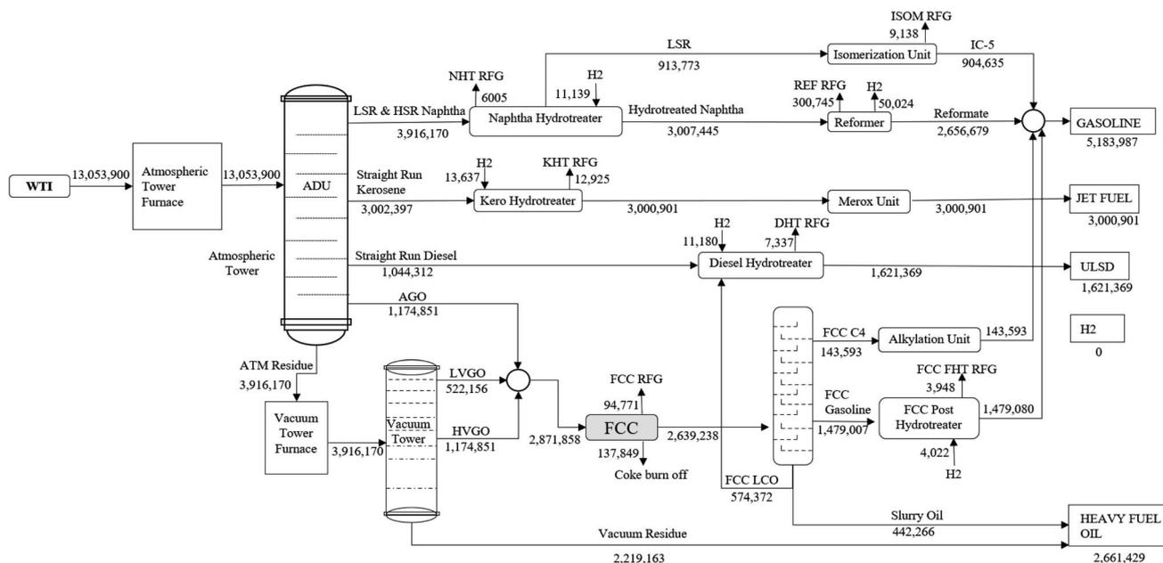
Fig. 2 Process mass flow in a traditional medium configuration refinery. The figure includes all the processes a crude oil undergoes to turn into commercial-grade fuels. The mass flow is also displayed for each process unit and all mass balances are shown in kg per day. This configuration mainly consists of an FCC as the upgrader. The final products are gasoline, jet fuel, ULSD, heavy fuel oil, and RFG that are reused for heating in the refinery.
