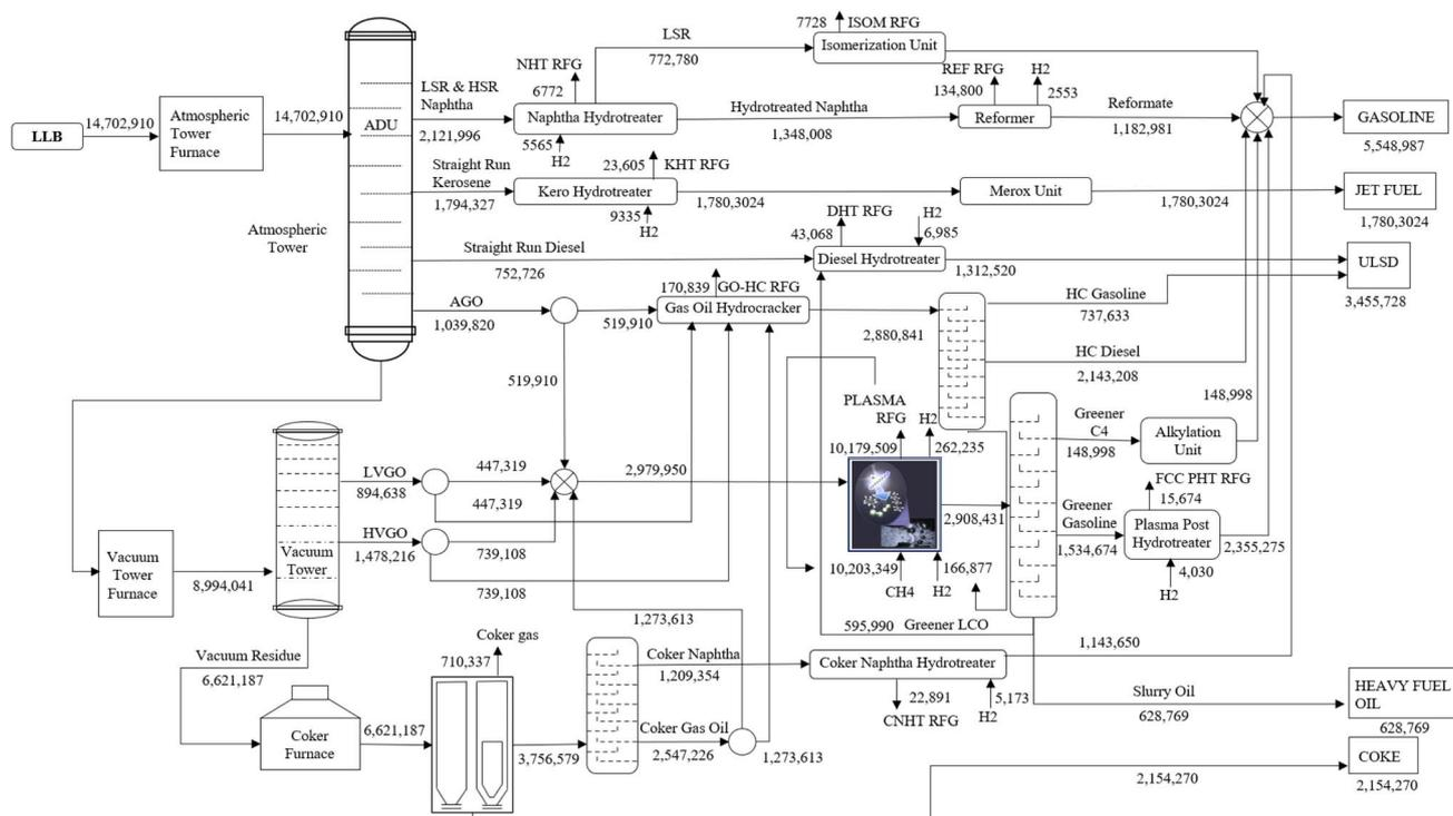
Fig. 5 Process mass flow diagram for a traditional deep conversion FCC and GO-HC coking 100 000 bbl per day capacity refinery with the FCC replaced by PPT. In this configuration, the FCC is also replaced by the PPT but the coker and hydrotreater remain unchanged.
