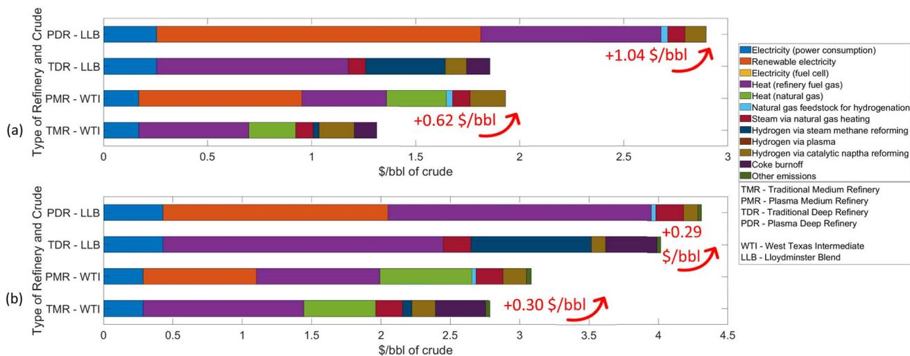
Fig. 7 (a) Comparison of energy cost with tax by using process units in different refinery scenarios. (b) Includes the carbon tax at a rate of \$0.05 per kg  $\text{CO}_{2\text{eq}}$  from the GHG emissions in addition to the energy cost. Adding a carbon tax reduces the cost difference to 10%.
