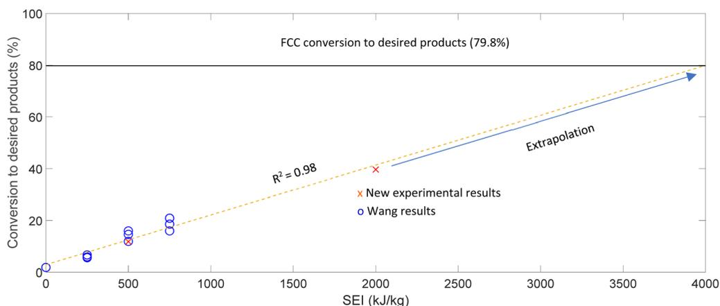
Fig. 1 SEI vs. overall conversion with new experimental results alongside Wang's prior results showing linear performance up to  $2000 \text{ kJ kg}^{-1}$  and extrapolated to  $4000 \text{ kJ kg}^{-1}$ . In an FCC, typically 79.8% of the feed is converted and the projected overall conversion for  $4000 \text{ kJ kg}^{-1}$  is similar to that of FCC.
