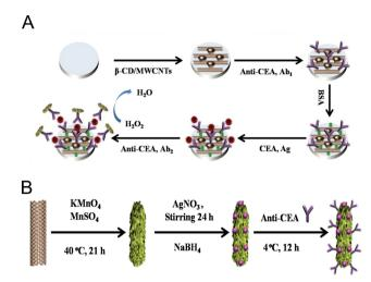
**Fig. 6** (A) Synthesis process of the label of a secondary antibody. (B) Schematic representation showing the fabrication process of the immunosensor. Reproduced from ref. 130 with permission from Elsevier, copyright [2017]. <sup>130</sup>
