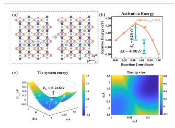
Fig. 5 (a) Structure diagram of the initial and final states of Li<sup>+</sup> hopping. (b) The activation energy calculated using the NEB for asymmetric ion hopping in  $Li_{0.125}$ FePO<sub>4</sub>, and (c) potential energy surface based on the Hamiltonian model (left) and its top view (right) for ion transport and electron transfer.
