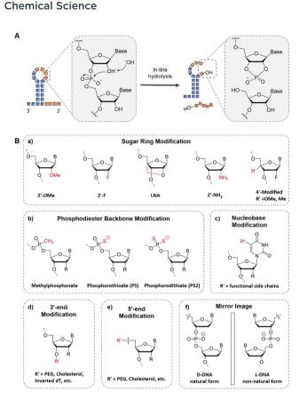
Fig. 3 The chemical modification of aptamers for improved stability. (A) The mechanism for RNA thermal instability.65 (B) The chemical modification in different sites of aptamers: (a) the sugar ring modification, (b) phosphodiester backbone modification, (c) nucleobase modification, and (d and e) end modification. (f) The chiral form of DNA. R represents -H for DNA and -OH for RNA.
