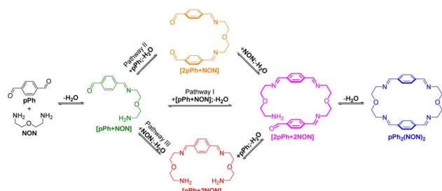
Scheme 2 Stepwise [2 + 2] imine condensation processes showing the intermediates on the way to the formation of the imine-based dynamic covalent macrocycle pPh_2(NON)_2 .
