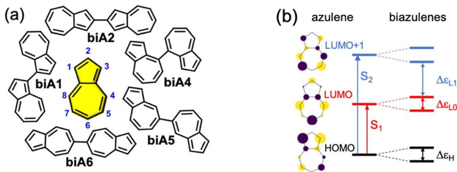
Fig. 2 (a) Molecular structures of azulene (yellow) and symmetrical biazulenes (**biA1**–**biA6**). (b) Hückel-type molecular orbital diagram for azulene and biazulenes. Vertical arrows indicate orbital transitions for  $S_1$  and  $S_2$  states in azulene. Double arrows indicate orbital gaps in biazulenes.
