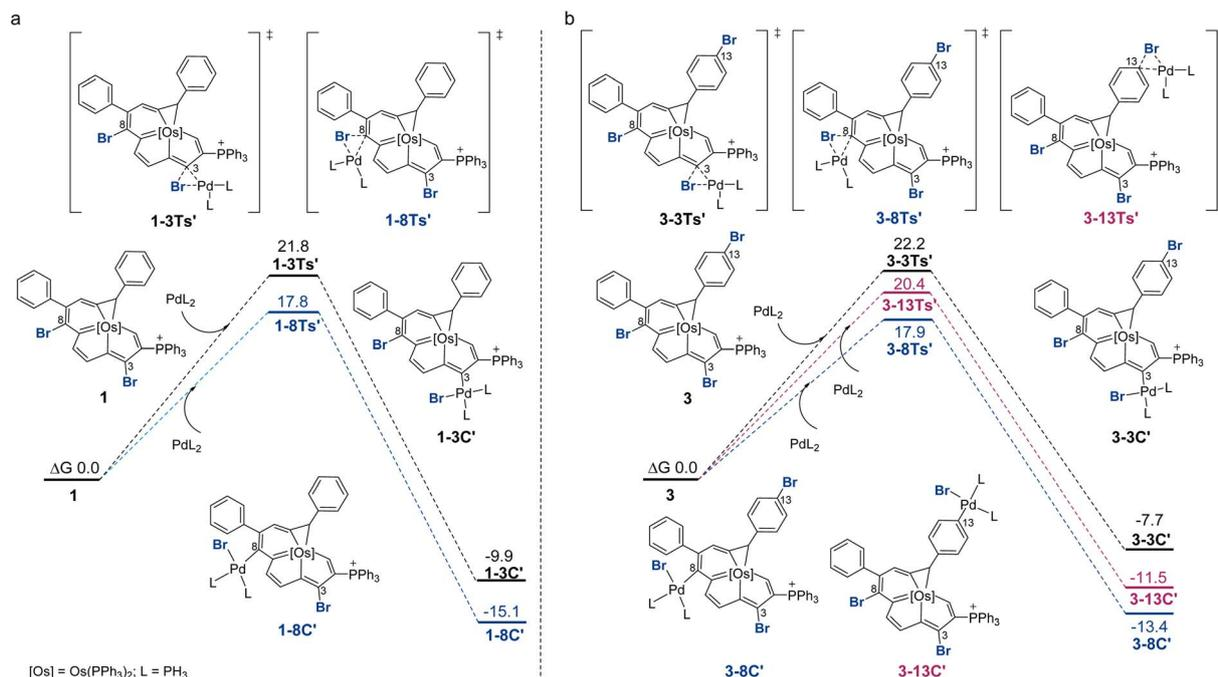
Fig. 2 DFT-computed Gibbs free energy profile for the oxidative addition steps. (a) Reaction between **1** and  $\text{PdL}_2$  at C3 and C8. (b) Reaction between **3** and  $\text{PdL}_2$  at C3 or C8 or C13,  $\text{L} = \text{PH}_3$ . All energies were computed at the level B3LYP-D3/def2-TZVP/PCM(o-DCB)//B3LYP/6-31G(d)(SDD for Os, Br, P), and are given in  $\text{kcal mol}^{-1}$ .
