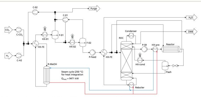
Fig. 8 Flowsheet of the heat integrated MeOH and DME synthesis plant producing DME from CO<sub>2</sub> and H<sub>2</sub>.
