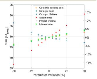
Fig. 7 Sensitivity analysis of economic parameters on the NCC of process P4 with C400 and crude MeOH feed (case B).
