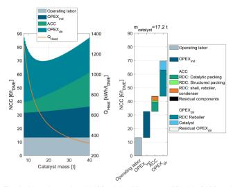
Fig. 4 Heat demand and NCC of the RD process P2 with C400 and pure MeOH feed in dependence of the catalyst mass in the RDC broken down into ACC, OPEX<sub>ind</sub>, and OPEX<sub>dir</sub> (left) as well as detailed cost breakdown at the cost optimum (right).
