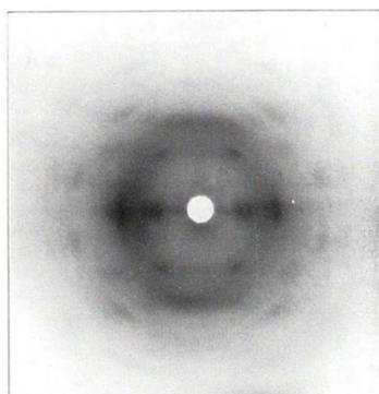
Fig. 7 The first published fibre diffraction pattern of NC with DoN of 12.6%, derived from nitration of ramie plant fibres. Reproduced with permission from ref. <sup>68</sup> with permission from John Wiley and Sons, copyright 1927.
