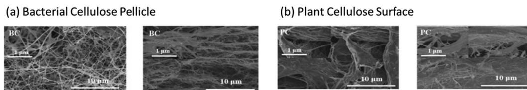
Fig. 4 Scanning electron microscopy (SEM) images of (a) a bacterial cellulose pellicle and (b) plant cell wall surface of cotton cellulose. Images reproduced from ref. <sup>36</sup> with permission from MDPI, copyright 2019.
