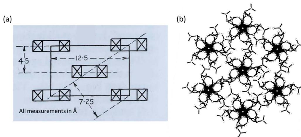
Fig. 9 Crystallographic models of NC proposed by (a) Miles in 1955 (orthorhombic) and (b) Happey *et al.* in 1978 (monoclinic, showing the now disputed five-fold axis). Illustrations reproduced from (a) ref. 47, copyright Imperial Chemicals Industry 1955 and (b) ref. 70 with permission from Elsevier, copyright 1978.
