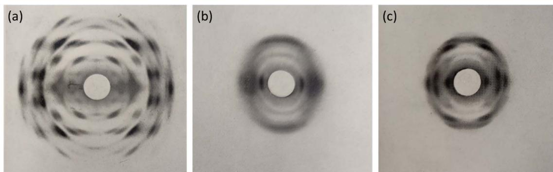
Fig. 8 X-ray diffraction patterns of (a) a ramie cellulose fibre, compared with (b) with di-substitution NC and (c) tri-substitution NC. Diffraction patterns reproduced from ref. <sup>45</sup>, copyright 1955.
