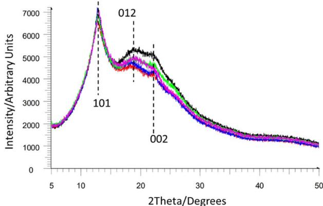
Fig. 10 Multiple overlapping NC powder diffraction patterns from ref. <sup>74</sup> reproduced with permission from Fraunhofer ICT, copyright 2014, with Miller index planes marked from indexing of NC by Miles *et al.* from ref. <sup>47</sup>.
