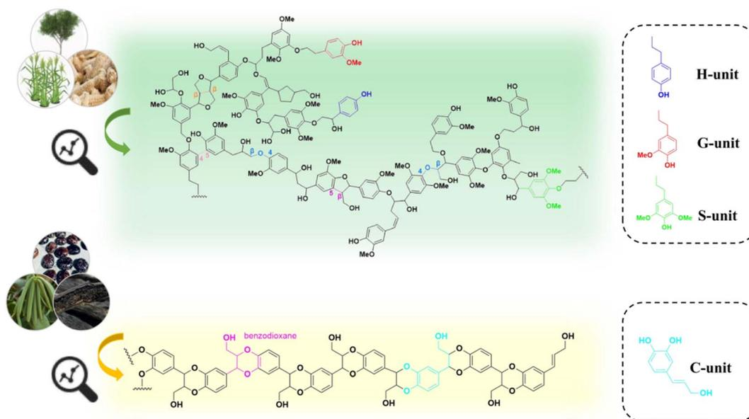
Fig. 1 Proposed structure of H/G/S lignin versus C-lignin revealed by NMR analysis.<sup>15</sup>
