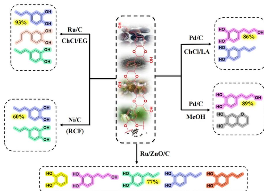
Fig. 3 Product composition and major monomer product selectivity during catalysis of C-lignin with different metal catalysts.<sup>16,24,43</sup>
