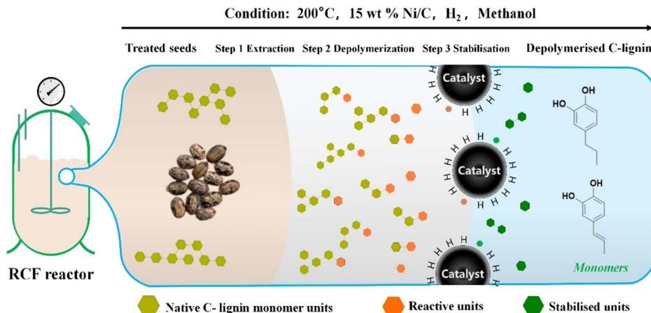
Fig. 4 Reductive catalytic fractionation (RCF) process of C-lignin.<sup>16</sup>
