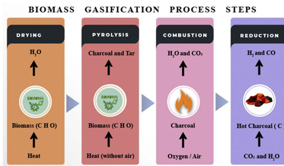
Fig. 3 Steps involved in the biomass gasification process.
