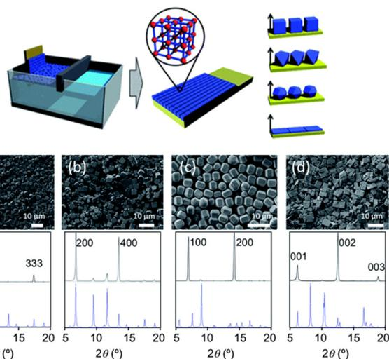
**Fig. 14** Scheme of the formation of oriented MOF layers by Langmuir–Blodgett. SEM images and corresponding out-of-plane XRD patterns of (a) octahedral HKUST-1, (b) cubic HKUST-1, (c)  $[\text{Al}_{12}\text{O}(\text{OH})_{18}(\text{H}_2\text{O})_3(\text{Al}_2(\text{OH})_4)(\text{BTC})_6]_n$ , and (d)  $[\text{Cu}_2(\text{BDC})_2(\text{bpy})]_n$ . Adapted with permission from ref. 103. Copyright 2012, Royal Society of Chemistry.
