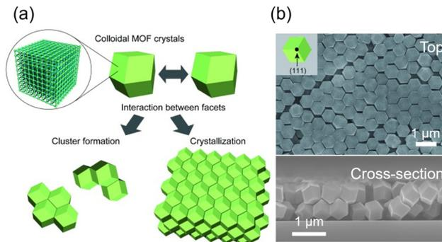
**Fig. 19** (a) Scheme of the interaction between ZIF-8 crystal facets driven by capillary forces and van der Waals interactions. (b) SEM images of top view (top) and cross-sectional view (down) of assembled ZIF-8 particles in  $\langle 111 \rangle$  direction parallel to the out-of-plane direction of Si substrates. Adapted with permission from ref. 107. Copyright 2012, Wiley-VCH.
