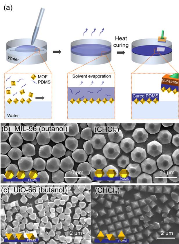
**Fig. 16** (a) Scheme of preparation of oriented MOF–PDMS films. (b) SEM images of oriented (b) MIL-96–PDMS films and (c) UiO-66–PDMS films prepared using butanol (left) and  $\text{CHCl}_3$  (right) as a casting solvent. Adapted with permission from ref. 101. Copyright 2021, American Chemical Society.
