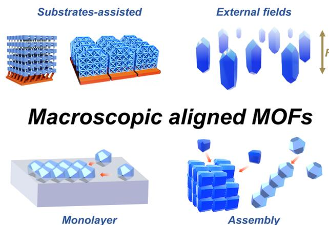
**Fig. 1** Schematic illustration of a variety of methods for preparing macroscopic aligned MOFs.
