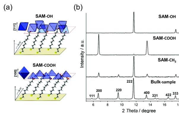
**Fig. 5** (a) Schematic illustration of [111] oriented HKUST-1 crystals with  $-\text{OH}$  SAM and [100] oriented HKUST-1 crystals with the  $-\text{COOH}$  SAM in the film. (b) XRD patterns of bulk and oriented films of HKUST-1 depending on the SAM functional groups. Adapted with permission from ref. 78. Copyright 2007, American Chemical Society.
