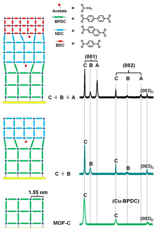
**Fig. 6** Schematic diagram depicting the step-by-step hetero-epitaxial growth of SURMOFs with a significant lattice mismatch, accompanied by XRD patterns illustrating the orientation of MOFs at each step. Adapted with permission from ref. 81. Copyright 2014, American Chemical Society.
