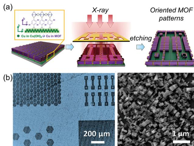
**Fig. 4** (a) A schematic illustration of the patterning of oriented MOF films *via* photolithography. (b) Optical image of micropatterned  $\text{Cu}_2[(\text{Br}_2\text{BDC})_x(\text{BDC})_{1-x}]_2\text{DABCO}$  oriented film on  $\text{Cu}(\text{OH})_2$  (left) and SEM image of oriented MOFs in the unexposed area to X-ray (right). Adapted with permission from ref. 75. Copyright 2023, Wiley-VCH.
