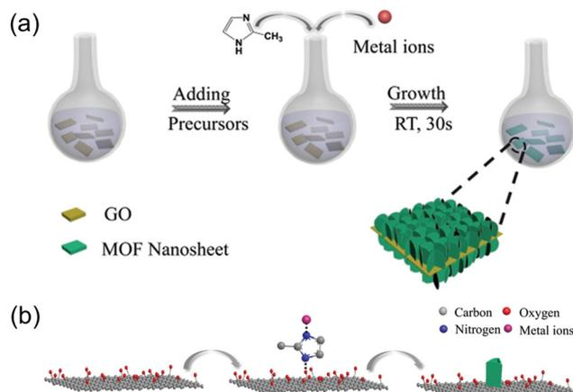
**Fig. 7** Schematic illustrations of (a) the synthesis for ZIF-67 nanosheets on GO substrate, as well as (b) the process of achieving vertically oriented nanosheets. Adapted with permission from ref. 82. Copyright 2020, Wiley-VCH.
