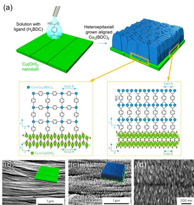
Fig. 3 (a) A schematic illustration inducing the heteroepitaxial growth of Cu<sub>2</sub>(BDC)<sub>2</sub> on 2D substrate of Cu(OH)<sub>2</sub> by reacting H<sub>2</sub>BDC solution with Cu(OH)<sub>2</sub>. SEM images of (b) 2D substrate of Cu(OH)<sub>2</sub> and epitaxially grown Cu<sub>2</sub>(BDC)<sub>2</sub> film on Cu(OH)<sub>2</sub> with (c) low and (d) high magnification. Adapted with permission from ref. 74. Copyright 2017, Springer Nature.
