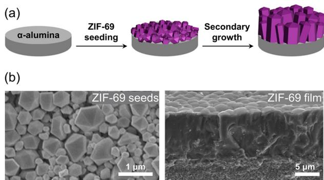
Fig. 2 (a) Schematic illustration of the process for synthesizing an oriented ZIF-69 film on an  $\alpha$ -alumina substrate by seeding ZIF-69 crystals and subsequent secondary growth. (b) SEM image of ZIF-69 seeds on the substrate (left) and cross-section of the oriented ZIF-69 film grown through secondary growth (right). Adapted with permission (part of figures) from ref. 72. Copyright 2011, Elsevier.
