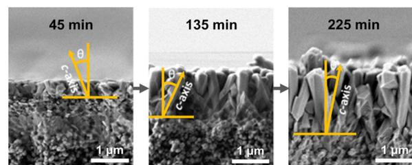
**Fig. 9** SEM images depending on different reaction times representing the extent of secondary growth of ZIF-7 in the out-of-plane direction with a tilted way from ZIF-7 nanocrystals on an alumina substrate. Adapted with permission from ref. 85. Copyright 2010, Wiley-VCH.
