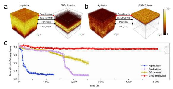
Fig. 9 (a) The spatial distribution of I<sup>-</sup> in the aged Ag and CNG devices. (b) The spatial distribution of Ag<sup>-</sup> and Cu<sup>-</sup> in the aged Ag and CNG devices. (c) The operational stability of the encapsulated Aq, Au, sprayed graphene (SG), and CNG-10 devices at the MPP under one sun illumination. Reproduced with permission.<sup>38</sup> Copyright 2022, Nature Publishing Groups.
