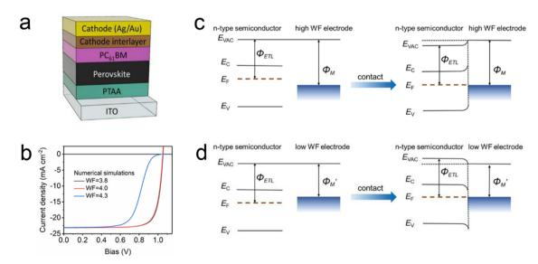
Fig. 2 (a) p-i-n device structure with cathode interlayer. (b) Numerical simulations of J-V curves based on different counter electrode work functions. Illustration of the band bending in the condition of (c) a high work function electrode and (d) a low work function electrode as the cathode. Reproduced with permission. 51 Copyright 2021, American Chemical Society Publications
