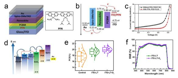
Fig. 8 (a) n-i-p device structure with a cathode interlayer PFN. (b) Energy level alignment and (c) J-V curves of devices with and without cathode interlayer modified electrode. Reproduced with permission. 92 Copyright 2017, Elsevier B.V. Publications. (d) Energy level alignment, (e) PCE statistics and (f) external quantum efficiency (EQE) of n-i-p solar cells with corresponding low-temperature processed ITO (LT-ITO) interlayer. Reproduced with permission.93 Copyright 2023, Wiley.
