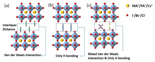
Fig. 1 Crystal structures of the three 2D perovskites. (a) RP phase, (b) DJ phase, and (c) ACI phase.
