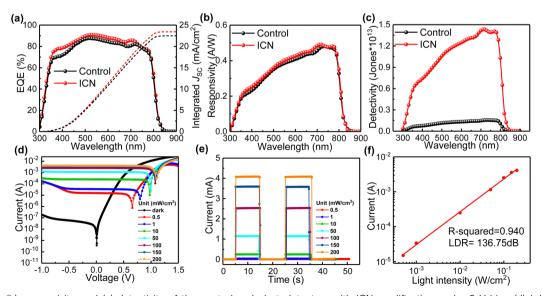
Fig. 5 (a) EQE, (b) responsivity, and (c) detectivity of the control and photodetectors with ICN modification under 0 V bias. (d) I-V curves of the photodetector with ICN modification under different light intensities. (e) I-T curves of the photodetector with ICN modification under various light intensities under 0 V bias. (f) Power-dependent photocurrent under 0 V bias for the photodetector with ICN modification.
