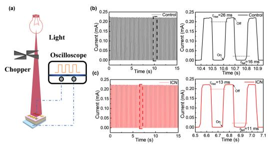
Fig. 6 (a) A schematic diagram of the light response speed test of self-powered photodetectors. The photocurrent response curves of (b) the control and (c) ICN-modified photodetectors under a 760 nm light source, respectively. The corresponding rise and decay times from the enlarged photocurrent response curve of photodetectors are shown on the right side.
