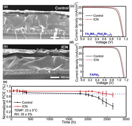
Fig. 3 Cross-sectional SEM images of the (a) control and (b) the ICN-modified devices. J-V curves of the champion control and ICN-modified PSCs based on (c)  $FA_xMA_{1-x}Pb(I_vBr_{1-v})_3$  and (d)  $FAPbI_3$ , two kinds of the photoactive layer. (e) Normalized PCE values of PSCs under ambient conditions with  $RH = 35 \pm 5\%$
