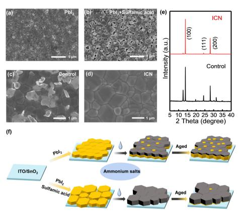
Fig. 1 Top-view SEM images of (a) the bare Pbl<sub>2</sub> film and (b) the Pbl<sub>2</sub> film with sulfamic acid modification. Top-view SEM images of (c) the control perovskite film and (d) the perovskite film with ICN modification. (e) XRD patterns of the perovskite films with and without ICN modification. (f) Schematic diagram of the two-step spin-coating method of perovskite active layers with and without sulfamic acid-based ICN strategy modification.
