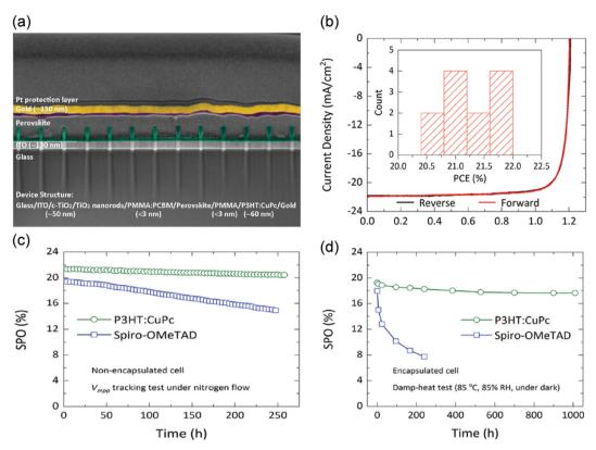
Fig. 10 (a) Cross-sectional SEM image, (b) J-V performance and (c) SPO of nonencapsulated cells based on P3HT:CuPc and spiro-OMeTAD HTL measured by Vmpp tracking under continuous 1 Sun illumination intensity. (d) SPO of encapsulated cells based on P3HT:CuPc and Spiro-OMeTAD HTL. Reproduced with permission. 131 Copyright 2021, Science.
