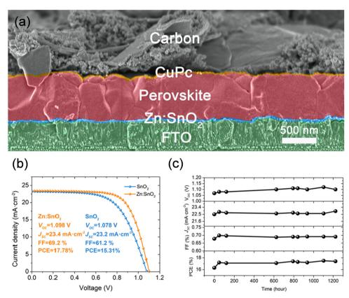
Fig. 2 (a) High-resolution cross-sectional SEM image of the carbon-based planar-structured PSC, (b) J-V curves of the best-performing PSC with SnO<sub>2</sub> or Zn-doped  $SnO_2$  as the ETM, (c) and evolution of the J-V parameters of the Zn-doped  $SnO_2$ -based devices stored in the ambient air with a relative humidity of  $\sim$  20%. Reproduced with permission. <sup>64</sup> Copyright 2019, Elsevier.
