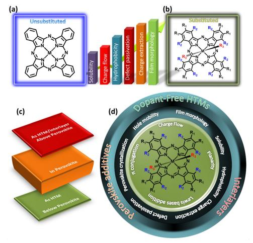
(a) Unsubstituted Pc, (b) substituted Pc, (c) Pc applications in different layers of PSCs and (d) design strategies linking the important parameters of PSCs.
