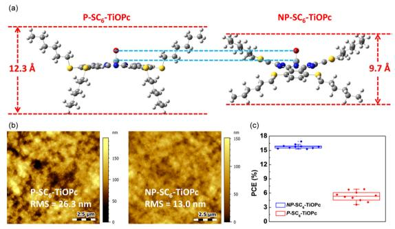
Fig. 8 (a) DFT results of the side view of the P-SC<sub>6</sub>-TiOPc- and NP-SC<sub>6</sub>-TiOPc-optimized ground state geometry (Gaussian 09 optimization with DFT B3LYP/6-31g(d)). (b) AFM images of P-SC<sub>6</sub>-TiOPc deposited and NP-SC<sub>6</sub>-TiOPc deposited on perovskite. (c) PCE statistics of devices fabricated from the same batch. Reproduced with permission. 103 Copyright 2019, ACS.
