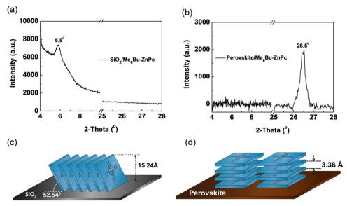
Fig. 7 GIXRD patterns of Me<sub>6</sub>Bu–ZnPc deposited on (a) SiO<sub>2</sub> and (b) perovskite (thin film thickness of  $\sim$  60 nm). Molecular orientation model of Me<sub>6</sub>Bu– ZnPc deposited on (c) SiO<sub>2</sub> and (d) perovskite. Reproduced with permission. <sup>100</sup> Copyright 2019, Wiley
