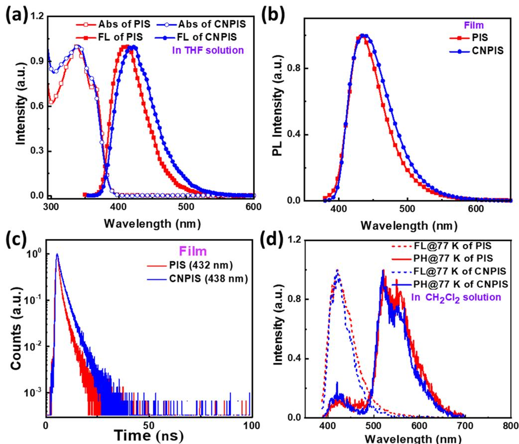
Fig. 1 (a) UV-vis absorption and emission spectra of **PIS** and **CNPIS** in dilute THF solution (10  $\mu$ M) at room temperature. (b) Emission spectra of **PIS** and **CNPIS** thin films. (c) Transient PL decay spectra of **PIS** and **CNPIS** thin films. (d) Low-temperature fluorescence and phosphorescence spectra of **PIS** and **CNPIS** in the dichloromethane solution.
