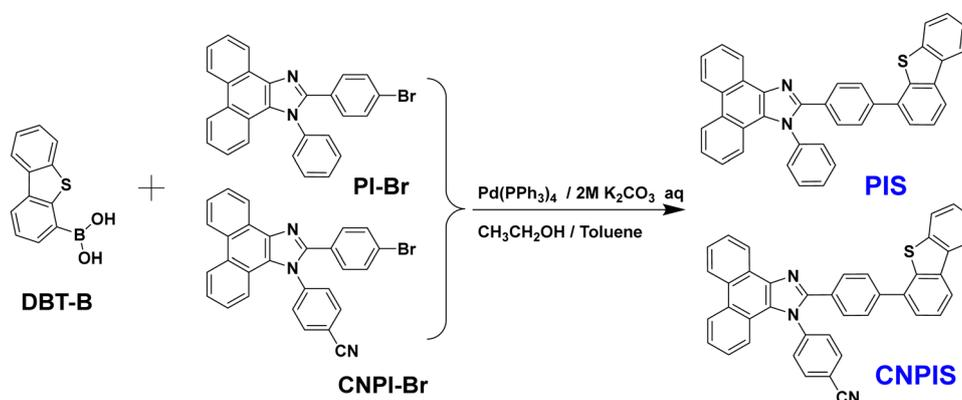
Scheme 1 The chemical equations for the synthesis of **PIS** and **CNPIS**.
