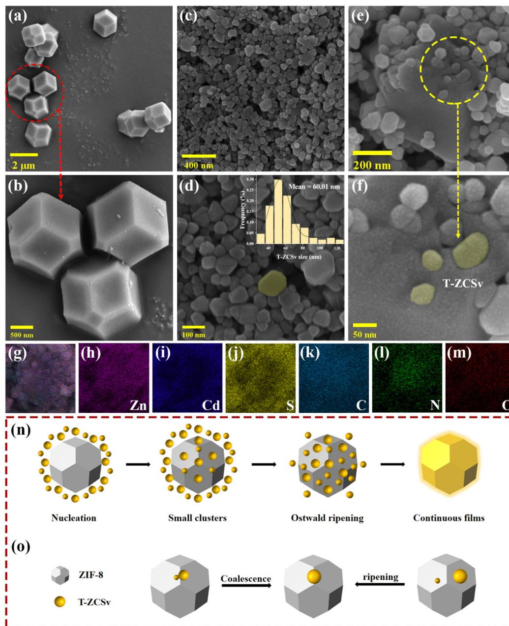
**Fig. 1** SEM images of ZIF-8 (a and b), T-ZCSv and the particle size distribution plot (c and d), ZIF-8@T-ZCSv (1300 mg) (e and f); the EDS element mapping of ZIF-8@T-ZCSv (1300 mg) (g–m); the model of the Ostwald ripening process (n) and comparison of ripening and coalescence (o).
