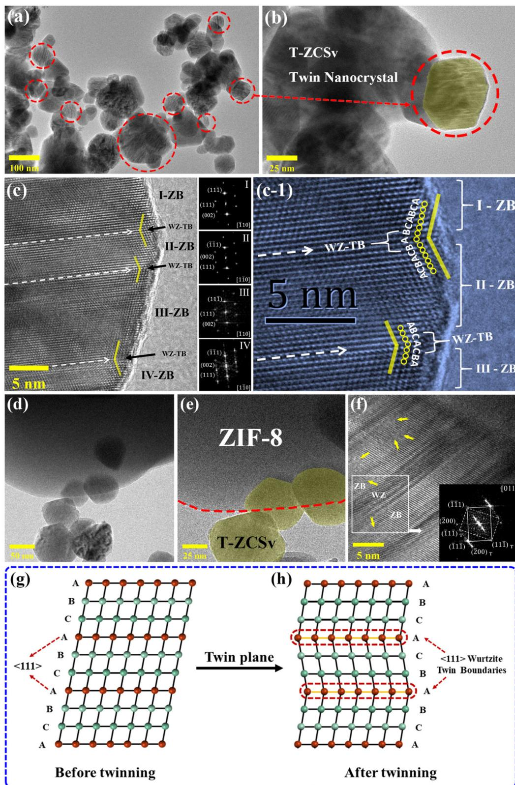
**Fig. 2** TEM images of T-ZCSv (a–c) and ZIF-8@T-ZCSv (1300 mg) (d–f) at different magnifications. The corresponding structural model of the twinning nanocrystal (g and h).
