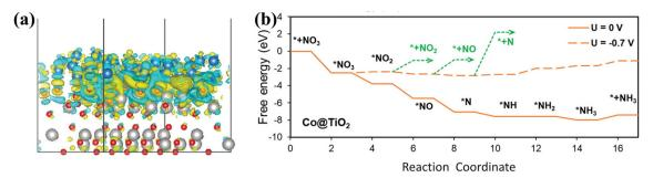
Fig. 11 (a) Mapping of the electron density difference. (b) Free energy diagram for  $NO_3^-$  conversion on  $Co@TiO_2$  copied with permission. 102 Copyright 2023, John Wiley and Sons.
