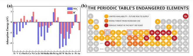
Fig. 5 (a) Adsorption energies for NO<sub>3</sub><sup>-</sup> species and protons on different metals copied with permission.<sup>59</sup> Copyright 2022, Elsevier. (b) The predicted elemental content of the periodic table within the next 100 years (gray represents high abundance) copied with permission.<sup>60</sup> Copyright 2021. Elsevier.
