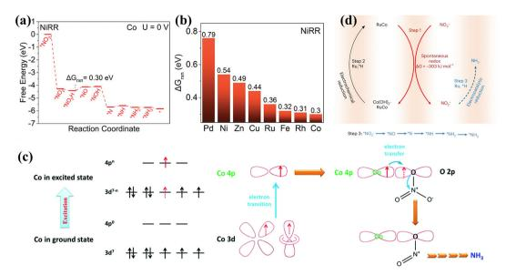
Fig. 9 (a) The Gibbs energy diagram of  $NO_3^-$  reduction on the Co surface. (b)  $\Delta G_{\rm rxn}$  on different metals copied with permission. 82 Copyright 2022, John Wiley and Sons. (c) Mechanism of NO<sub>3</sub><sup>-</sup> reduction on CoP copied with permission. 85 Copyright 2022, Royal Society of Chemistry. (d) The three-step relay route of Ru<sub>x</sub>Co<sub>v</sub> alloy copied with permission. <sup>87</sup> Copyright 2023, Springer Nature.
