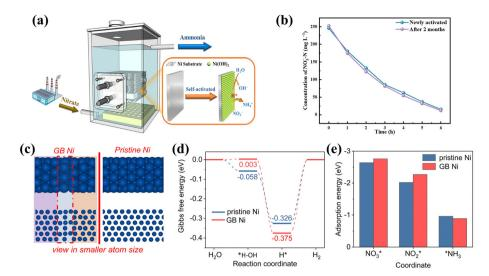
Fig. 10 (a) Diagram of an electrochemical reactor on the pilot scale and (b) comparison of initial NO<sub>3</sub><sup>-</sup> reduction performance and that after two months copied with permission. 92 Copyright 2021, American Chemical Society. (c) The simulated structure, (d) Gibbs free energy diagrams of the HER and (e) adsorption energies of important N-containing species on GB Ni and pristine Ni copied with permission.<sup>93</sup> Copyright 2023, Royal Society of Chemistry.
