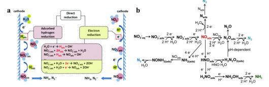
Fig. 2 (a) The proposed direct and indirect pathways of nitrate electroreduction. (b) The electron-mediated pathway of nitrate electroreduction copied with permission.<sup>38</sup> Copyright 2021, Royal Society of Chemistry.
