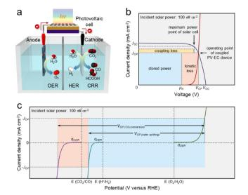
Fig. 1 The principles of photovoltaic-electrochemical (PV-EC) device. (a) Schematic of PV-EC cell. (b) The generalized current density-voltage (J-V) diagram (2-electrode measurement) of a directly coupled PV-EC device. Reproduced from ref. 13. Copyright 2013 PNAS. (c) The generalized J-V diagrams (3-electrode measurement) of anode and cathode for electrochemical reactions (water splitting and CO<sub>2</sub> conversion).
