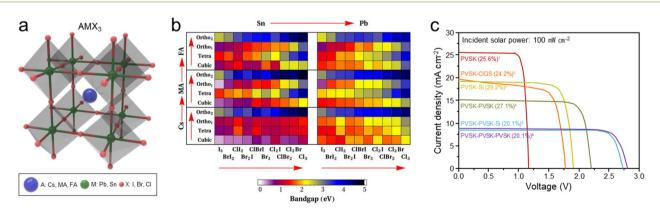
Fig. 3 Halide perovskite-based solar cells. (a) General crystal structure (AMX<sub>3</sub>) of the halide perovskite. (b) Calculated band gaps of halide perovskites with different composition and phase. Reproduced from ref. 43. Copyright 2014 AIP Publishing. (c) J-V curves of various halide perovskite tandem solar cells with benchmarked power conversion efficiencies (PCE). Benchmark list: (1) ref. 55, (2) ref. 46, (3) ref. 54, (4) ref. 53, (5) ref. 52, (6)
