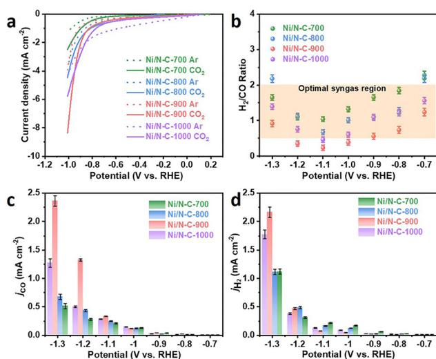
Fig. 3 (a) Linear sweep voltammetric (LSV) curves of various samples in CO<sub>2</sub> and Ar-saturated 0.1 M KHCO<sub>3</sub> solution. (b) Dependence of the H<sub>2</sub>/CO ratio on the applied potentials of Ni/N-C-700, 800, 900 and 1000. Partial current densities of CO (c) and H<sub>2</sub> (d).
