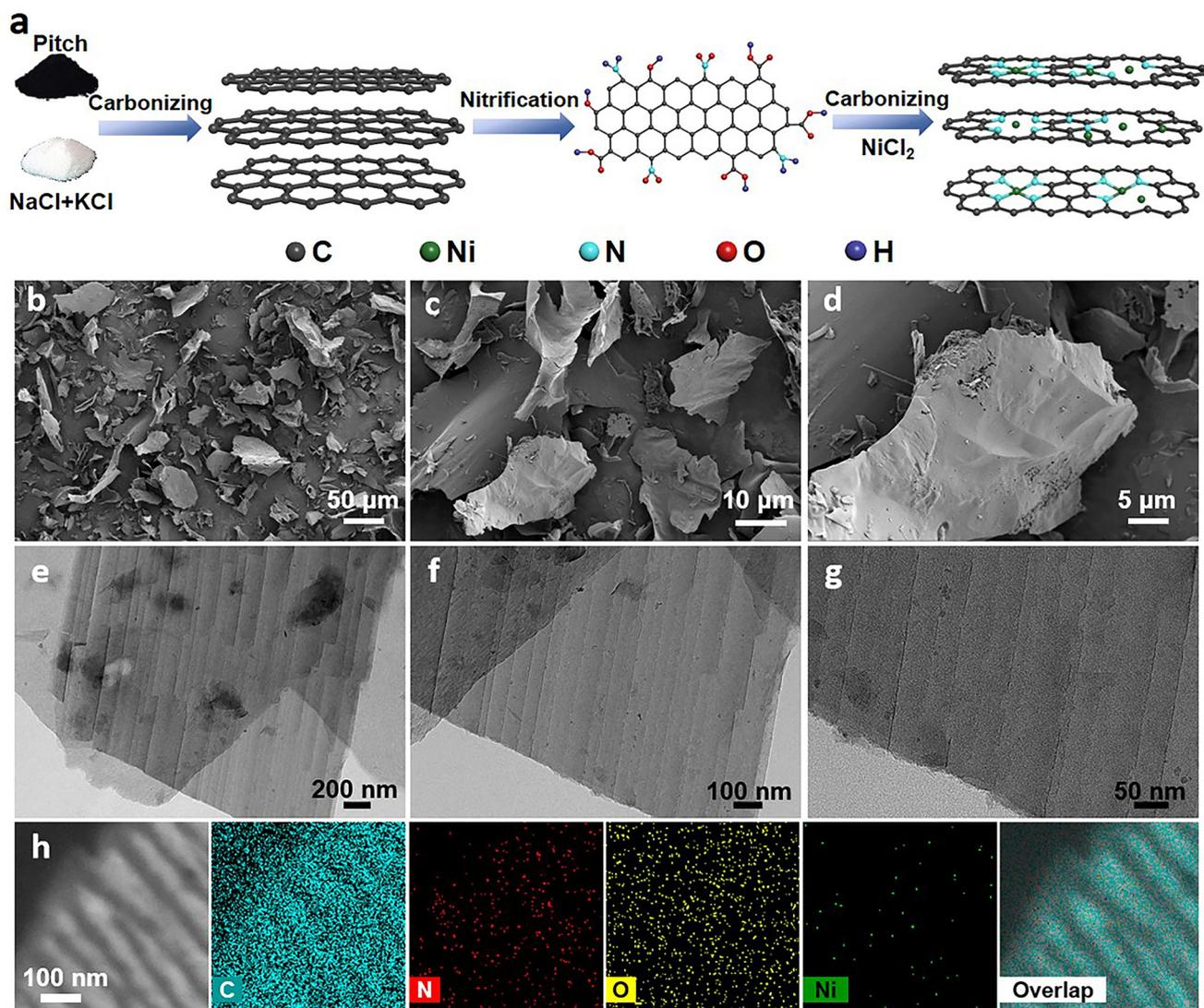
**Fig. 1** (a) Schematic diagram of the synthetic procedure of the Ni/N-C catalysts. (b–d) SEM, (e–g) TEM and (h) EDS mapping images of Ni/N-C-900.
