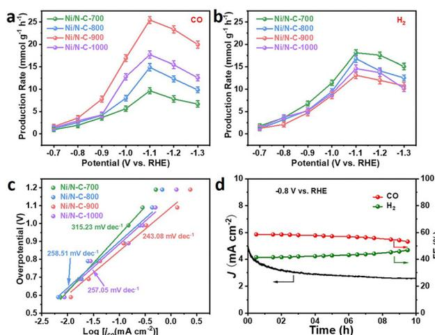
**Fig. 4** (a) CO and (b) H<sub>2</sub> production rates of Ni/N-C catalysts at different applied potentials. (c) Tafel plots based on  $j_{\text{CO}}$  of the Ni/N-C catalysts in CO<sub>2</sub>-saturated 0.1 M KHCO<sub>3</sub> solution. (d) Long-term stability test of Ni/N-C-900 at  $-0.8$  V vs. RHE for 10 h.
