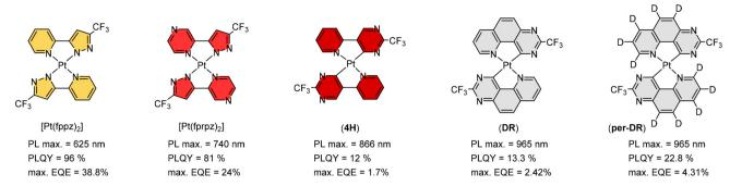
Scheme 3 Representative Pt(II) complexes showing strong solid-state aggregation and efficient emissions in saturated red and NIR regions.
