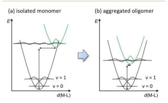
**Scheme 4** Schematic potential energy diagrams for square planar Pt(III) emitters (a) as isolated molecules and (b) after aggregation and formation of intimate Pt...Pt interaction.
