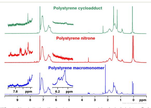
Fig. 6 <sup>1</sup>H NMR spectra of the cycloadduct formed from the polystyrene macromonomer and nitrone functionalized polystyrene. The disappearance of peaks in the region of 7.8 ppm to 8.4 ppm in polystyrene nitrone and 5.9 ppm to 6.3 ppm in the polystyrene macromonomer for the polystyrene cycloadduct confirms the utilization of the nitrone functionality in the 1,3-dipolar cycloaddition reaction.
