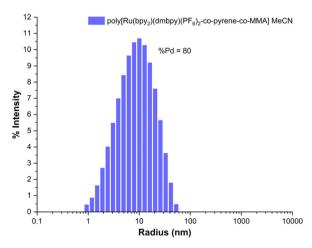
Fig. 4 Dynamic light scattering (DLS) of poly[Ru(bpy)<sub>2</sub>(dmbpy)(PF<sub>6</sub>)<sub>2</sub>-co-pyrene-co-MMA] in (left) dimethyl sulfoxide (DMSO) and (right) acetonitrile (MeCN).
