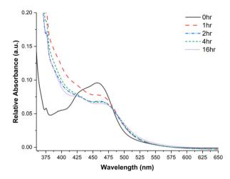
Fig. 8 UV-Vis spectra in DMSO obtained during the reaction of 4-bromobenzontirile and N-methylpyrrole demonstrating progressive decrease in the fidelity of the Ru(11) complex. The spectra were collected at identical concentrations.
