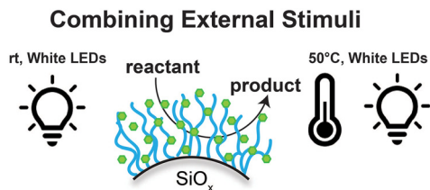
Fig. 1 Illustration of the overall idea of combining both thermal and light responsive features on a surface.
