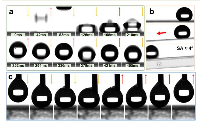
Fig. 7 Analysis of dynamic behaviour of water droplets. (a) Images demonstrate the repeating bounce behavior of a 15 µL water droplet on a horizontally placed spray-coated glass. (b) The SA test result of AFSR/EP@n-SiO<sub>2</sub> coatings with a 15 µL water droplet. (c) The test process of non-stacking property of AFSR/EP@n-SiO2 coatings towards the water droplet using a contact angle measuring instrument.
