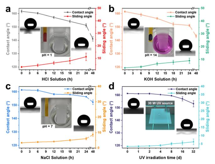
Fig. 6 Contact angle and sliding angle of AFSR/EP@n-SiO<sub>2</sub> coatings immersed in various harsh solutions with (a) pH = 1, HCl, (b) pH = 14, KOH, phenolphthalein indicator was added for color indication, and (c) pH = 7, NaCl (10 wt%) for a long time. (d) Hydrophobicity test of the prepared surface under 30 W ultraviolet light source.
