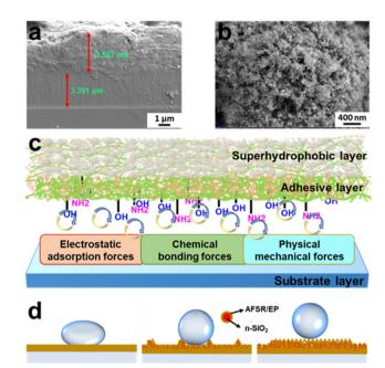
(a) FE-SEM image of double-layer cross-section surface of glass sample with coating. (b) High power FE-SEM image of the AFSR/EP@n-SiO<sub>2</sub> superhydrophobic coating surface at nanoscale magnifications. (c) Schematic diagram of the layered structure of the AFSR/EP@n-SiO<sub>2</sub> superhydrophobic coating and the mechanism of strong bonding properties, and (d) simplified wetting model of three rough coating structures and different hydrophobic mechanism diagrams.
