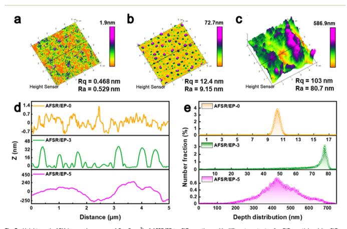
Fig. 3 Height-mode AFM images (scan area of  $5 \times 5 \mu m^2$ ) of AFSR/EP@n-SiO<sub>2</sub> coatings with different contents of n-SiO<sub>2</sub> particles, (a) n-SiO<sub>2</sub> = 0 wt%, (b) n-SiO<sub>2</sub> = 3 wt%, and (c) 5 wt%, respectively. (d) AFM 3D images showing the cross-sectional micro profiles at 2.5 μm of the AFSR/EP@n-SiO<sub>2</sub> coating. (e) Statistical distribution of the height of the coating on the glass sheet substrate.
