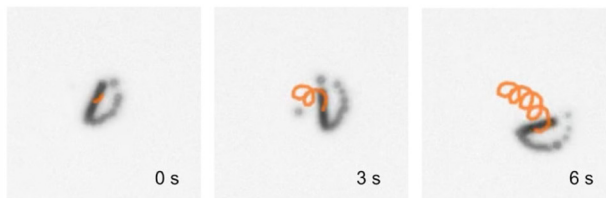
C Time lapse of \text{MnO}_2/\text{Lac} micromotor trajectories at 2 wt. % \text{H}_2\text{O}_2
