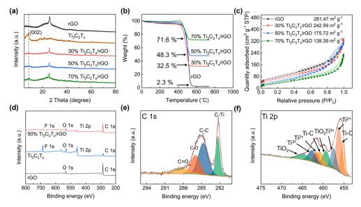
Fig. 2 (a) XRD patterns of rGO,  $T_{i3}C_2T_x$  and  $T_{i3}C_2T_x/r$ GO nanocomposites. (b) TGA curves of rGO and  $T_{i3}C_2T_x/r$ GO nanocomposites. (c)  $N_2$  adsorption/desorption isotherms of rGO and  $T_{i3}C_2T_x/r$ GO nanocomposites. (d) XPS survey spectra of rGO,  $T_{i3}C_2T_x$  and  $T_{i3}C_2T_x/r$ GO nanocomposites. (e) C 1s and (f) Ti 2p XPS spectra of  $T_{i3}C_2T_x/r$  nanocomposites.
