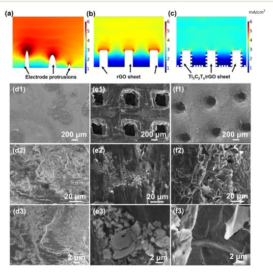
Fig. 4 Surface current density distribution simulated by COMSOL Multiphysics on (a) Cu, (b) 3D-printed rGO and (c) 3D-printed 50% Ti<sub>3</sub>C<sub>2</sub>T<sub>x</sub>/rGO electrodes. SEM images of (d) Cu, (e) 3D-printed rGO and (f) 3D-printed 50% Ti<sub>3</sub>C<sub>2</sub>T<sub>x</sub>/rGO electrodes after 100 cycles at 2 mA cm<sup>-2</sup> with 2 mA h  $cm^{-2}$ .
