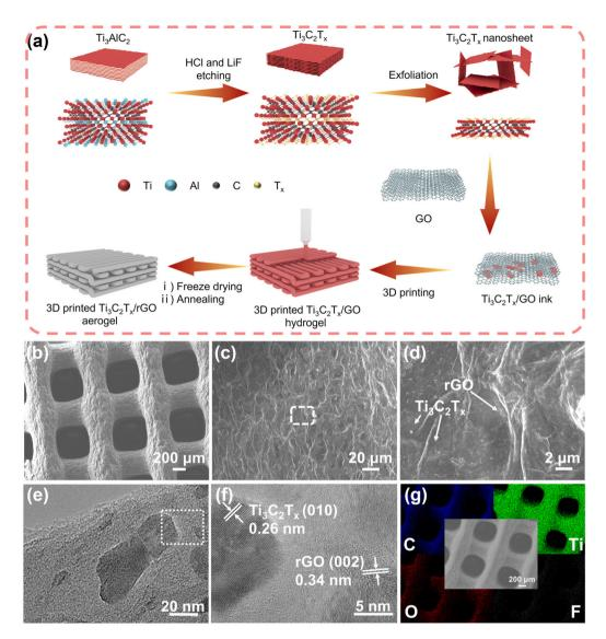
Fig. 1 (a) A schematic diagram of the preparation process of 3D-printed Ti<sub>3</sub>C<sub>2</sub>T<sub>x</sub>/rGO microlattice aerogel electrodes. (b–d) SEM and (e and f) TEM images of the 3D-printed 50% Ti<sub>3</sub>C<sub>2</sub>T<sub>x</sub>/rGO electrode. (g) SEM image of the 3D-printed 50% Ti<sub>3</sub>C<sub>2</sub>T<sub>x</sub>/rGO microlattice aerogel and the corresponding EDS elemental mapping.
