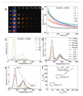
Fig. 3 (a) Afterglow photographs of CCCP:x%Mn (x = 0-20) crystals taken under UV excitation and at different times after the removal of the UV light. (b) Afterglow decay curves, and (c) TL curves of CCCP:x%Mn (x = 0-20). (d) The TL curves of CCCP:x%Mn obtained at various delay times from 1 min to 24 h. (e) The TL curves of CCCP:x%Mn recorded with preheating at various temperatures. (f) The x0 The TL curves of CCCP:x1 The TL curves of CCCP:x2 Mn.
