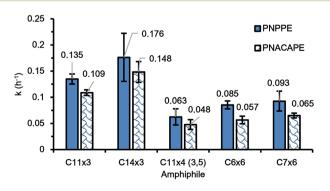
Fig. 4 Rate constants of PNPPE (blue, solid fill) and PNACAPE (blue, shingle pattern) depropargylation in presence of C11x3, C14x3, C11x4 (3,5), C6x6 and C7x6 metallic micelles.
