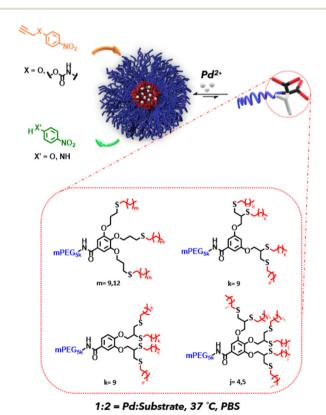
Fig. 1 Schematic illustration of Pd<sup>II</sup>-loaded micellar nanoreactors based on PEG-dendron amphiphiles with varied architectures for the depropargylation of substrates with different propargyl protecting groups.
