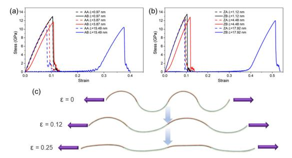
Fig. 5 The calculated stress-strain curves of the MoSSe/WSSe heterostructure superlattice with (a) armchair and (b) zigzag interfaces with different lengths L; (c) the side view of the structural evolution schematic for the AB MoSSe/WSSe heterostructure under uniaxial tension.
