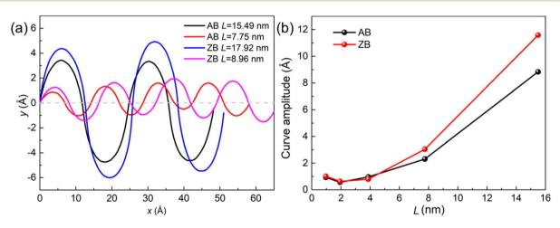
Fig. 3 (a) The fitted Fourier curve for the structural trajectory of the MoSSe/WSSe heterostructure superlattice and (b) the amplitude value of the Fourier curve versus L.
