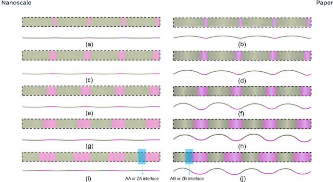
Fig. 2 The top and side views of optimized (a, c, e, g, and i) AA and (b, d, f, h, and j) AB Janus MoSSe/WSSe heterostructures with  $L_{\rm m}/L_{\rm n}$  as (a and b) 1/9, (c and d) 2/8, (e and f) 3/7, (g and h) 4/6, (i and j) 5/5, respectively.
