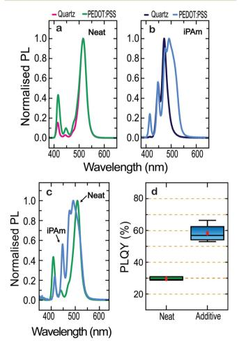
Fig. 2 Photoluminescence characteristic of  $\langle n \rangle$  = 2 thin films deposited on quartz and PEDOT of the (a) neat system (b) and the iPAm system, (c) comparison of both systems when deposited on PEDOT, and the (d) PLQYs of 12 samples of iPAm and neat thin films.
