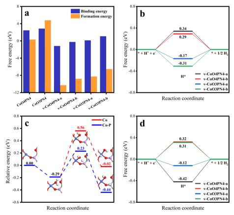
Fig. 6 (a) Binding energies and formation energies of CoO4PN4, CoO3PN4, v-CoO4PN4-a, v-CoO4PN4-b, v-CoO3PN4-a, and v-CoO3PN4-b. (b) H adsorption free energy at Co sites in v-CoO4PN4-a, v-CoO3PN4-a, and v-CoO3PN4-b. (c) Relative free energy of water splitting reaction pathway on Co site and Co-P cooperation on v-CoO3PN4. (d) H adsorption free energy at P sites in v-CoO4PN4-a, v-CoO4PN4-b, v-CoO3PN4-a, and v-CoO3PN4-b.
