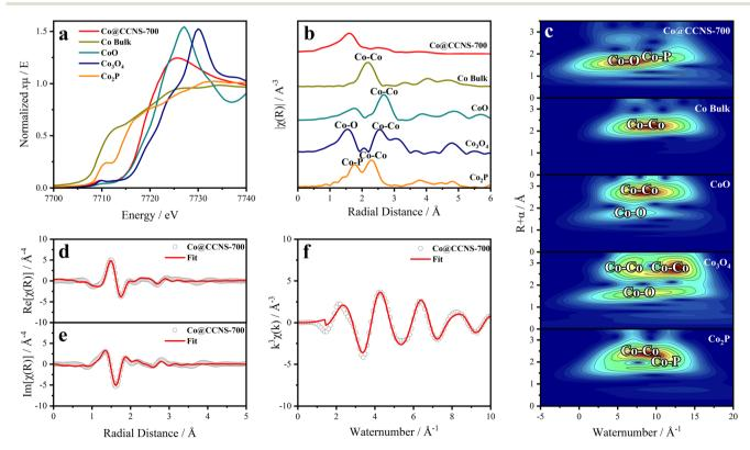
Fig. 5 (a) Normalized X-ray absorption near edge structure (XANES) spectra of cobalt k-edge in Co@CCNS-700. (b) Fourier transform and (c) wavelet transform on extended X-ray absorption fine structure (EXAFS) data of Co@CCNS-700. Fittings of (d) real part and (e) imaginary part of R-space and (f) k-space EXAFS plots of Co@CCNS-700.
