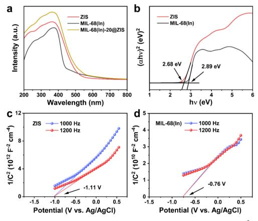
Fig. 5 Energy band structure. (a) UV-vis absorption spectra of ZIS, MIL-68(In) and MIL-68(In)-20@ZIS; (b) Tauc plots of  $(\alpha h \nu)^2$  vs. photon energy  $(h \nu)$  for ZIS and MIL-68(In); M-S plots of (c) ZIS and (d) MIL-68(In).
