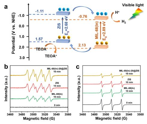
Fig. 6 The photocatalytic mechanism of MIL-68(In)@ZIS. (a) schematic illustration of charge transfer paths for MIL-68(In)@ZIS; EPR spectra of (b) DMPO  ${}^{\circ}O_2^{-}$  and (c) TEMPO  ${}^{+}$  for ZIS, MIL-68(In) and MIL-68(In)-20@ZIS.
