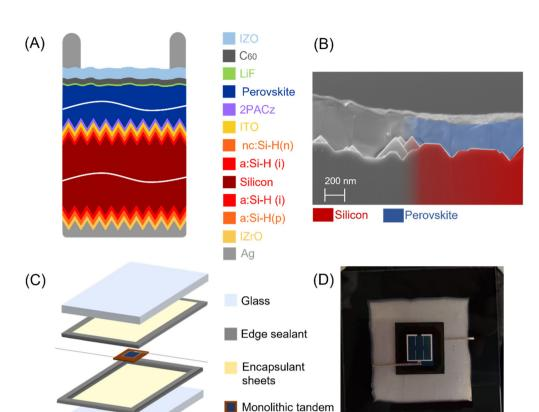
Fig. 1 (A) Schematic representation of the textured monolithic perovskite/silicon tandem solar cell. (B) Cross-sectional scanning electron microscopy image of the tandem solar cell. (C) Minimodule components representation. (D) Top view of the tandem minimodule.
