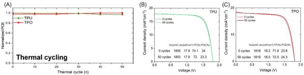
Fig. 5 (A) Power conversion efficiency trend during 50 cycles of TC test. (B) and (C) Comparison between the J-V curves before and after the TC test in the case of two minimodules encapsulated with TPU and TPO, respectively.
