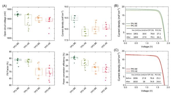
Fig. 2 J-V related parameters of monolithic perovskite/silicon tandem solar cell before and after encapsulation with TPU and TPO (A). Comparison between the J-V curves of the best devices before and after encapsulation with (B) TPU and (C) TPO.
