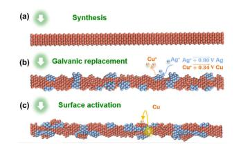
Fig. 3 (a) Starting CuNWs. (b) Galvanic replacement on the surface. (c) Surface activation through in situ formation of CuAq assemblies during the electrochemical CO<sub>2</sub>RR. Reproduced with permission from ref. 57. Copyright 2021, Springer.
