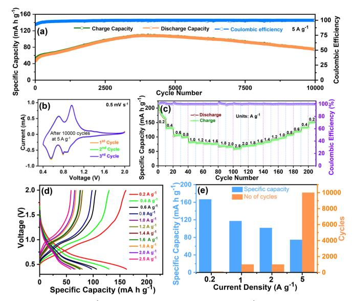
Fig. 5 Cycling performance at 5 A  $g^{-1}$ , (b) CV curves after the cycling test (at a scan rate of 0.5 mV  $s^{-1}$ ), (c) rate performance, (d) voltage profile curves at different scan rates, and (e) specific capacity vs. current density of the O–CuVSe composite cathode.
