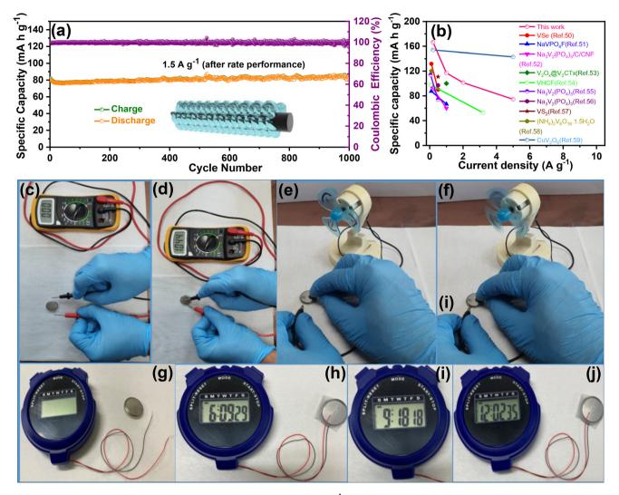
Fig. 6 (a) Cycling performance of the O-CuVSe composite cathode at 1.5 A  $g^{-1}$ . (b) Comparison of the electrochemical performances of the previously reported literature with the O-CuVSe composite cathode. (c and d) Photographic images of representing the OCV in the Zn/O-CuVSe composite battery. (e and f) Photographic images of the Zn/O-CuVSe composite battery powering a toy motor fan. (g-j) Photographic images of the Zn/O-CuVSe composite battery powering a digital watch.
