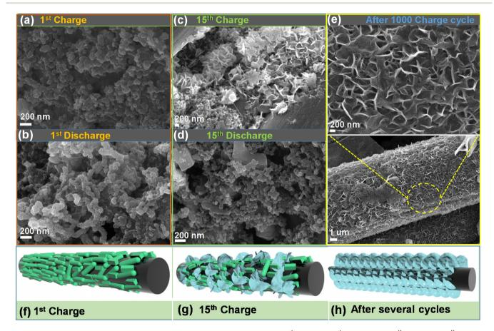
Fig. 8 FE-SEM images of the O-CuVSe composite cathode measured after the (a) 1st charge, (b) 1st discharge, (c) 15th charge, (d) 15th discharge, and (e) 1000 charge cycles. (f-h) Schematic illustration for the morphology change during the cycling process.
