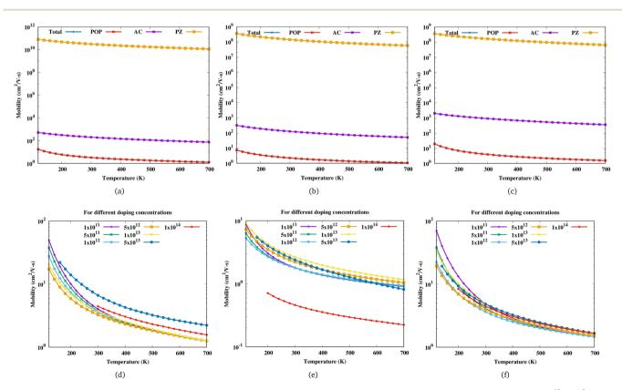
Fig. 3 Mobility of (a)  $Sc_2CF_2$ , (b)  $Sc_2CO_2$  and (c)  $Sc_2C(OH)_2$  as a function of temperature for an electron concentration of  $5 \times 10^{12}$  cm<sup>-2</sup> with the contributions of POP, acoustic and PZ scattering. Mobility of (d) Sc<sub>2</sub>CF<sub>2</sub>, (e) Sc<sub>2</sub>CO<sub>2</sub> and (f) Sc<sub>2</sub>C(OH)<sub>2</sub> as a function of temperature for different electron concentrations in cm<sup>-2</sup>
