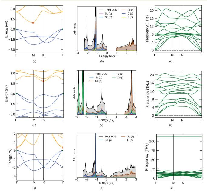
Fig. 1 Electronic band structures, density of states and phonon band structures of (a-c)  $Sc_2CF_2$  (first row), (d-f)  $Sc_2CO_2$  (second row) and (g-i)  $Sc_2C(OH)_2$  (third row). The y (vertical) scale of DOS plots are multiplied by 2, 2 and 5 factors for F, O and OH functional groups respectively. In the electronic band structure, the VBM and CBM are denoted by green and red points respectively.
