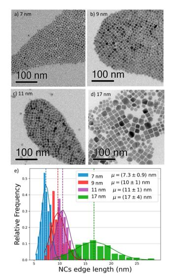
Fig. 1 (a-d) Bright field transmission electron microscopy (TEM) images of four different CsPbl<sub>3</sub> NCs, revealing their cubic shape and sizes of 7, 9, 11, and 17 nm. The solutions have low polydispersion and narrow size distribution. (e) Size distribution histogram of the imaged NCs (statistics: 200 per size), showing narrow distributions (±1 nm) for the smaller sizes, and a broader distribution ( $\pm 4$  nm) for the 17 nm NCs.
