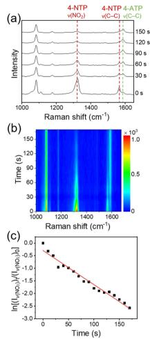
Fig. 3 (a) Time-dependent SERS spectra of 4-NTP and (b) corresponding color-coded intensity map of the SERS spectra obtained after the treatment of an aqueous solution of NaBH<sub>4</sub> onto the device. (c) Plot of the logarithm of the intensity of  $\nu(NO_2)$  peak relative to that of the initial stage versus the reaction time.
