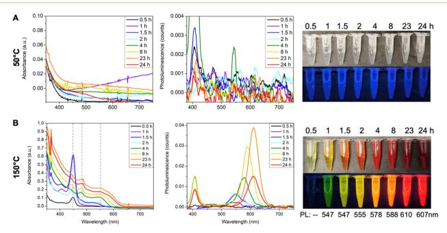
Fig. 5 Effect of temperature on CdTe MSC formation. The reactions at (A) 50 °C and (B) 150 °C are monitored by absorption, emission, and photos of aliquots under ambient light and UV light, respectively.
