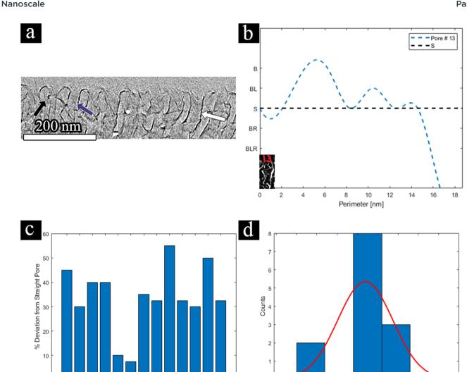
Fig. 6 TEM tomography analysis – (a) selective slice from the TEM tomography 3D data; the white arrow shows a Double-Wall Curved Bend pore (B), the black arrow shows a Single-Wall Bend left pore (BL), and the blue arrow shows a Straight pore (S), (b) a perimeter profile of a single porepore #13 at p=0 nm (inset), (c) deviation from a straight pore for 13 selected pores, (d) a histogram of the deviation from a straight pore.
