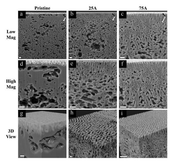
Fig. 3 (a-f) Cross-sectional SEM images and (g-i) reconstructed 3D volume of pristine membrane (a, d and g) and membrane modified with 3 cycles of AlO<sub>x</sub> SIS and 25 (b, e and h) or 75 cycles of AlO<sub>x</sub> ALD (c, f and i). Images d-f are higher magnifications of images a-c, respectively. The black arrows point to the highly ordered selective layer and the white arrows to the underneath supporting layer. All the scale bars are 200 nm.
