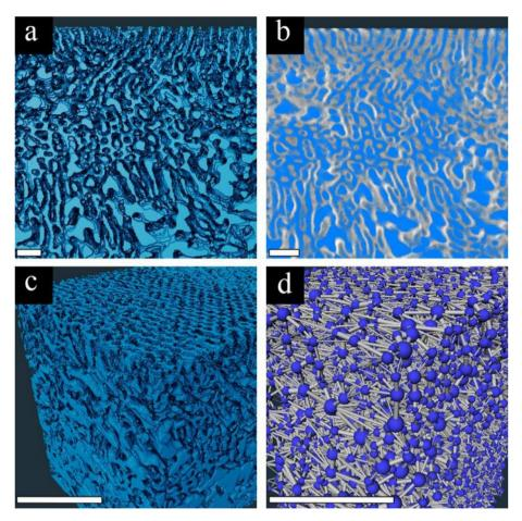
Fig. 4 Segmentation of the FIB-SEM tomography 3D volume: (a) cross-sectional view of the segmented data, (b) segmentation overlayed with the original data, (c) 3D view of segmented data, and (d) 3D pore network reconstruction performed by using Amira. All the scale bars are 200 nm.
