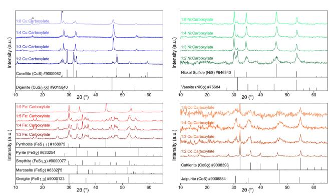
Fig. 1 pXRD of transition metal sulfides: copper sulfide (top left), nickel sulfide (top right), iron sulfide (bottom left), and cobalt sulfide (bottom right) Reflections from copper(I) thiocyanate denoted by \* (ICSD #24372)
