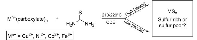
**Scheme 1** General synthesis of transition metal  $(M^{n+})$  sulfide nanoparticles to give either sulfur rich or sulfur poor phases.
