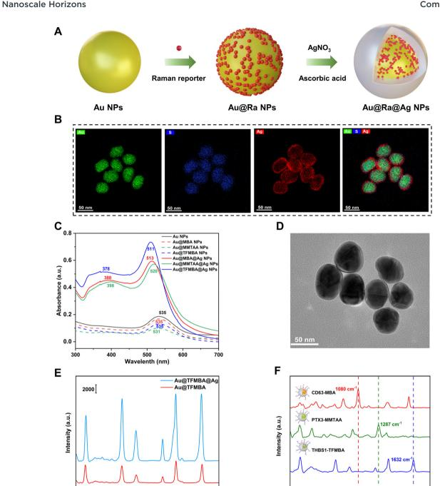
Fig. 1 Preparation and characterization of SERS nanotags. (A) The synthesis of Au@Ra@Ag NPs using Raman reporter molecules as anchors. (B) EDS mapping of Au@TFMBA@Ag NPs. (C) UV-vis absorption spectra of Au NPs, Au@Ras NPs, and Au@Ras@Ag NPs. (D) A TEM image of Au@TFMBA@Ag NPs. (E) SERS spectra of Au@TFMBA NPs and Au@TFMBA@Ag NPs in water. (F) SERS signals of Au@Ra@Ag NPs with antibody-Raman reporter pairs of CD63-MBA, PTX3-MMTAA, and THBS1-TFMBA.
