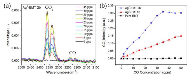
Fig. 4 (a) In situ IR spectra Ag-EMT-2b film by increasing the CO concentration from 2 to 50 ppm at RT. (b) The IR absorption intensities of CO<sub>2</sub> dependent on the amount of CO with pure EMT, Ag-EMT-1b, and Ag-EMT-2b films in the range of 2–50 ppm.
