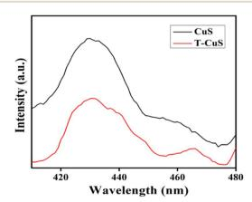
Fig. 7 Photoluminescence spectra of CuS and the T-CuS nanocomposite.
