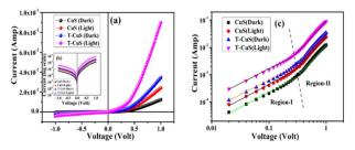
Fig. 10 (a) Current–voltage (I-V) plots, (b) log scale I vs. V curves and (c) log I–log V plot of the bare CuS and T-CuS composite-based Schottky diodes under dark and illumination conditions.
