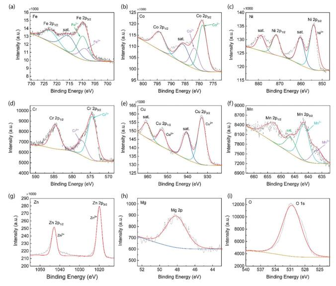
XPS analysis of 8-HEO NPs. (a) Fe 2p, (b) Co 2p, (c) Ni 2p, (d) Cr 2p, (e) Cu 2p, (f) Mn 2p, (g) Zn 2p, (h) Mg 2p, and (i) O 1s.
