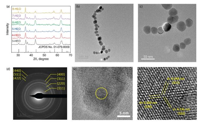
Fig. 3 (a) XRD patterns of HEO NPs with 3 elements to 8 elements. (b). STEM images of 8-HEO NPs. (c) SAED analysis of 8-HEO NPs to confirm the spinel crystal structure. (d-f) HRTEM of 8-HEO NPs.
